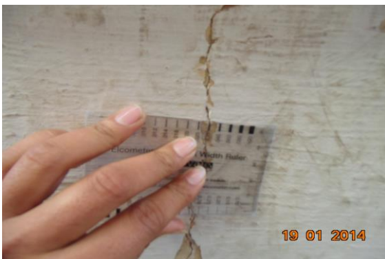
Photo 15A Inclined Crack on Wall No. 1 of , Police H.Q. First Floor, Part B, Approx. Width = 0.35mm, Approx. Length = 1m. Distance from Wall 4 = 3.2m, Height from Floor = 0.12m.
