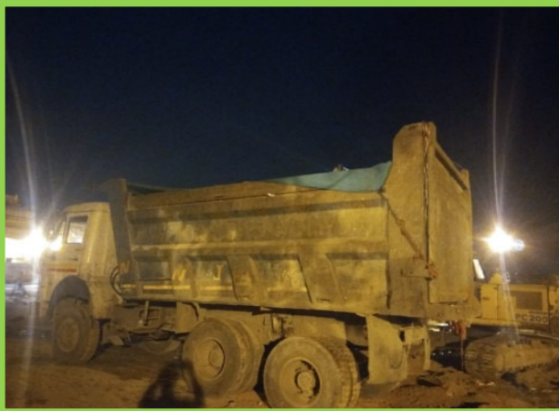
Loaded dumper properly covered by tarpaulin
