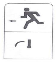
when viewed from inside. Concise operating instructions describing each motion necessary to unlatch and open the exit shall be displayed. These instructions shall be located within 150 mm of the release mechanism.
